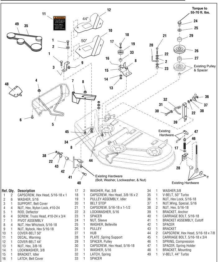
Figure 1. Contents of Turbo Installation Kit
